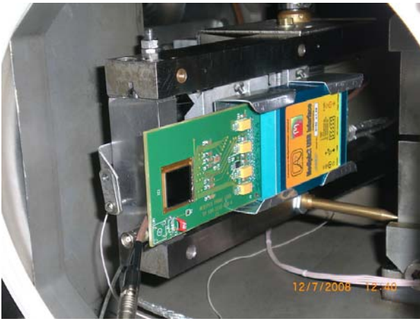
Fig. 1. Photo of TimePix mounted in a vacuum chamber on a moveable platform at the focal plane of the laser mass spectrometer.
