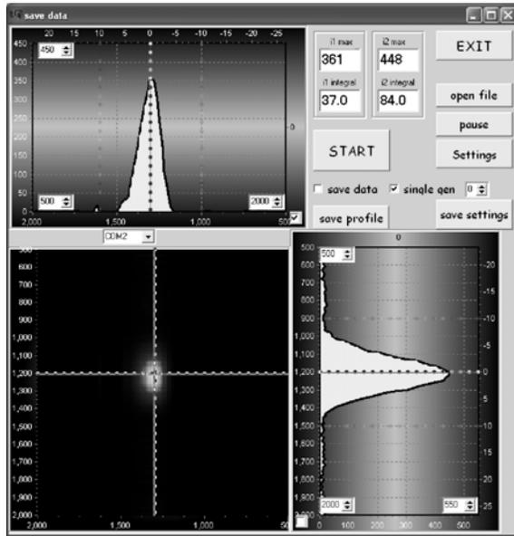
Fig. 2. An example of the  $^{11}\text{B}$  beam profile is displayed by the data acquisition software. The beam energy was 33 AMeV, beam intensity was  $1\ \mu\text{A}$ , measured under the pressure of  $2 \cdot 10^{-5}$  mbar. In the top-left and the bottom-right panels the dependences of  $I_1(U_1)$  and  $I_2(U_1)$  are displayed, respectively. In the bottom-left (central) panel 2D beam profile is shown.
