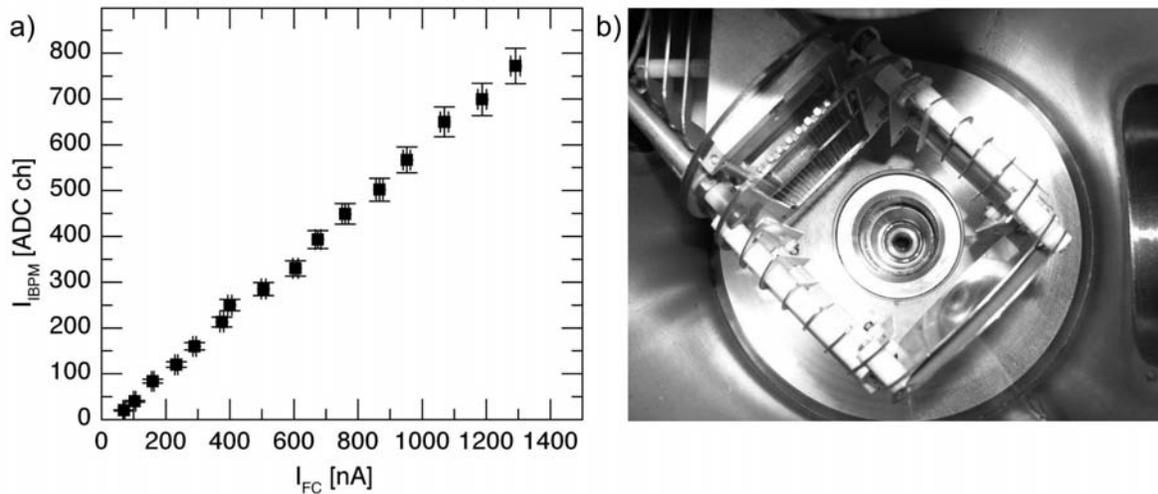
Fig. 3. a) Dependence of the ionization current  $I_{IBPM}$  (vertical axis) on the beam current measured by Faraday cup (horizontal axis). b) The location of the IBPM in front of the production target of the ACCULINNA separator. The round dark circle in the center of the picture is the target material.
