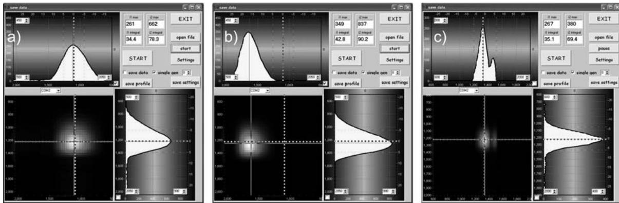
Fig. 4. a)  $^{11}\text{B}$  centered on the beam optical axis. b) The beam aligned on the border of the calibration frame, installed at the entrance of the diagnostic box, corresponding to a half width of the square hole in the frame ( $\sim 17$  mm). c) Example of the two beams profile for the different beam energies. Main peak corresponds to the nominal energy; the small peak corresponds to the beam coming at lower energy.
