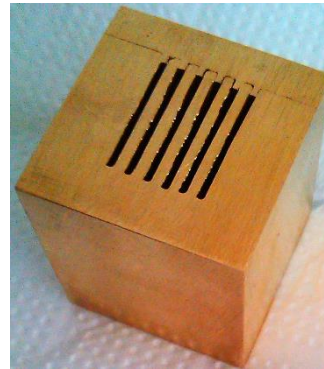
Fig. 2. Photo of the prototypes of the collimators for shaping mini-beam structures for the spatially fractionated hadron radiation therapy. See color Figure on journal website.
