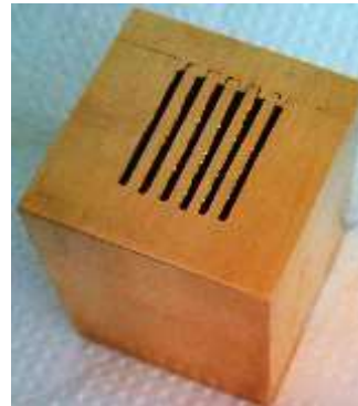
Fig. 2. Photo of the prototypes of the collimators for shaping mini-beam structures for the spatially fractionated hadron radiation therapy. See color Figure on journal website.
