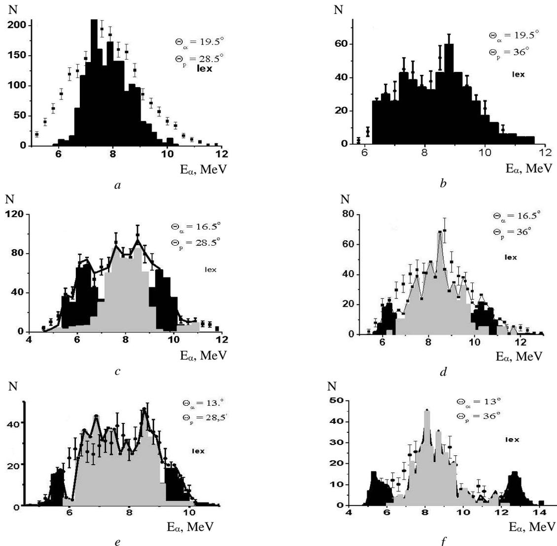
Fig. 2, (a - f). Projections of vertical strips of the two-dimensional ( $E_p \times E_\alpha$ ) spectra on the energy axes of alpha-particles for the first excited state of the  ${}^6\text{He}$  nucleus. Black dots – experimental data. Parameterizations by the Monte Carlo method: black columns – configuration “dineutron”, gray light columns – “cigar”. The solid black line – its sum.
