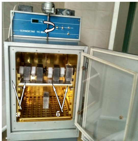
Fig. 3. Air bath oven with the device for exposure of ^{137}\text{Cs} contaminated blood samples: a – containers with samples; b – protective lead blocks.
