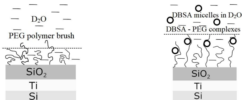
Fig. 5. Schematic representation of substrate layers with a polymer brush system in deuterated water ( left ), the formation of surfactant - polymer complexes in polymer brush systems ( right ).
